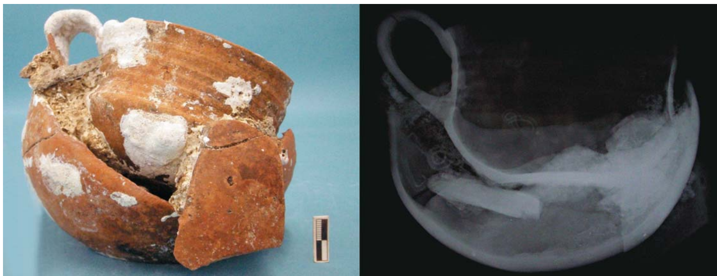
Figure 1. Pottery cluster that includes a carinated cup and other fragments before cleaning (left), and as shown in radiograph (right). The X-ray was taken using a Faxitron 43855A X-ray System (56 cm focus-to-film distance, 110 kV, 3 min, 3mA).
